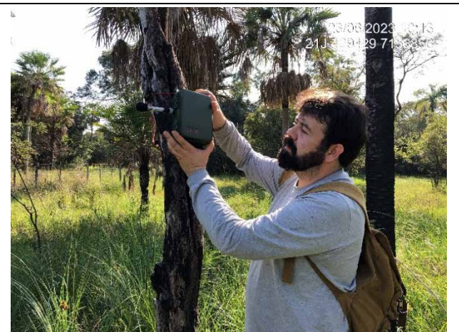
Photo 18: Detail of the Songmeter bioacoustic device installed for the detection of bats (Second Campaign).
