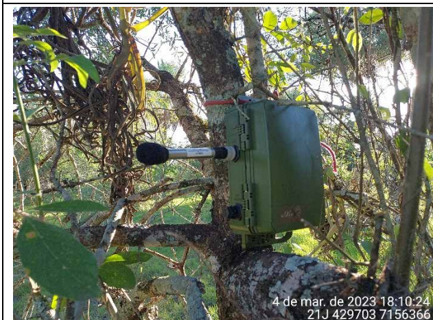
Photo 17: Detail of the Songmeter bioacoustic device installed for the detection of bats (First Campaign).
