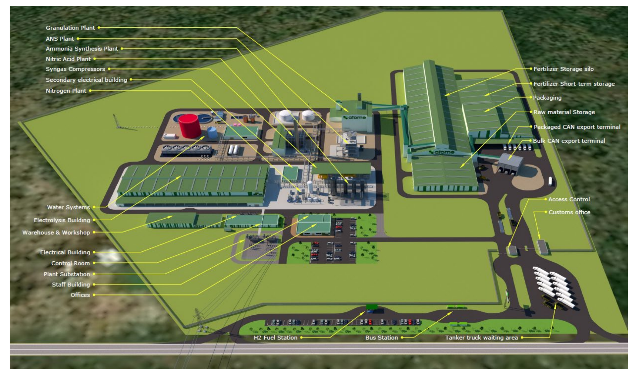
Preliminary plant design for 145MW Villeta green ammonia and calcium ammonium nitrate production facility
